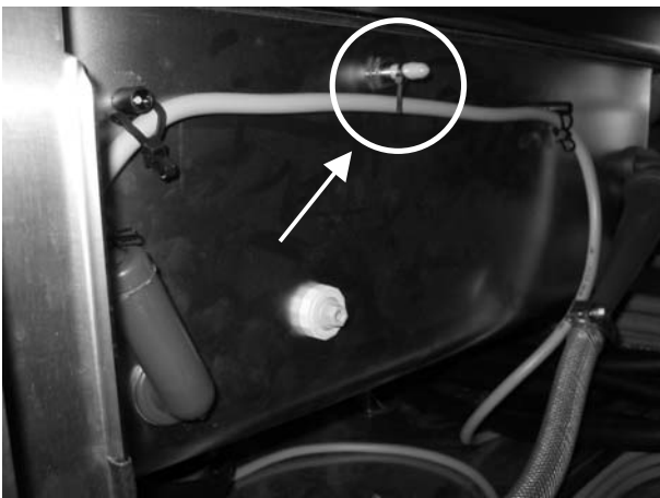
Fig.: Last main wash zone with dosing nipple for detergent
