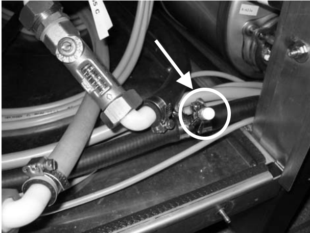
Fig.: Last main wash zone with dosing nipple for rinse aid
